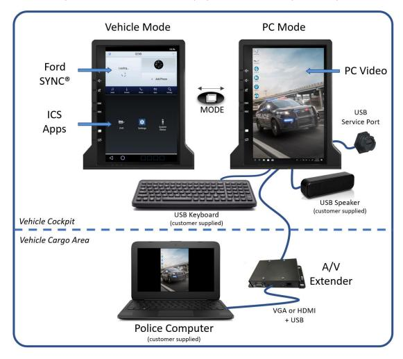
The ICS allows relocation of the police computer from the cockpit to the cargo area. The computer connects using standard HDMI/VGA and USB interfaces to an Audio/ Video Extender (AVX) which converges these standard interfaces into a single CAT6 cable that runs to the front of the vehicle and connects to the ICS screen.
