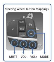
**Note:** The Police Interceptor 4 remappable latching switches are mapped to discrete output signals (wires) that can be used for controlling other equipment in the police car (See up-fitters guide).
