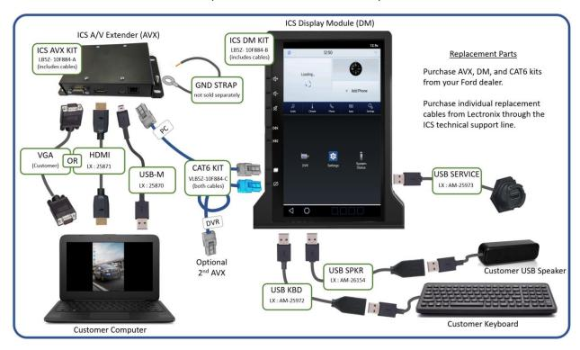
When the vehicle is delivered, the Display Module is already installed and any cables that connect to it are installed and left accessible to the customer to complete installation of equipment.
