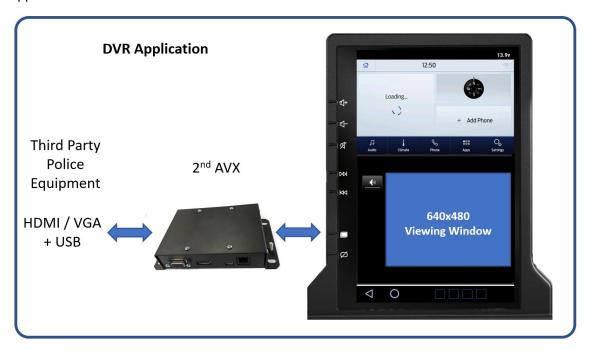
The user interacts with the connected equipment by touching within the viewing window. To the left of the viewing window is a MUTE button that provides a convenient way to enable and disable audio from the device.
