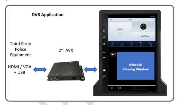
The user interacts with the connected equipment by touching within the viewing window. To the left of the viewing window is a MUTE button that provides a convenient way to enable and disable audio from the device.
